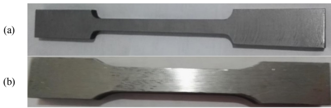
Fig. 3. Samples for (a) tensile testing and (b) fatigue testing
