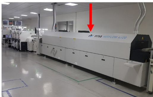
Fig. 3. In-line industrial reflow oven (dual-lane 14×2 zones) in SMT line
