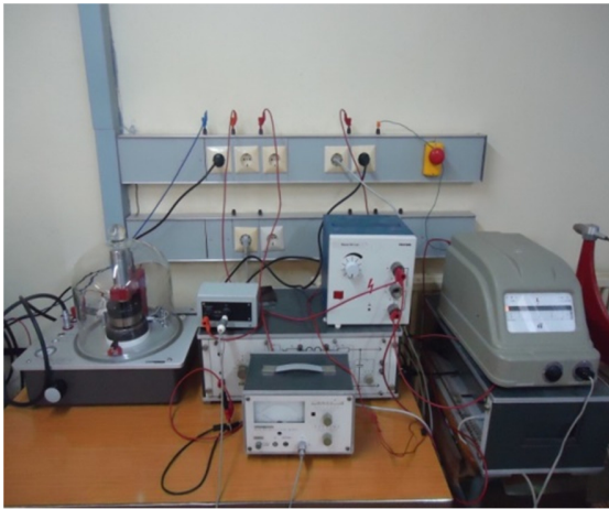
Fig. 1. Measuring circuit of the volume resistivity
