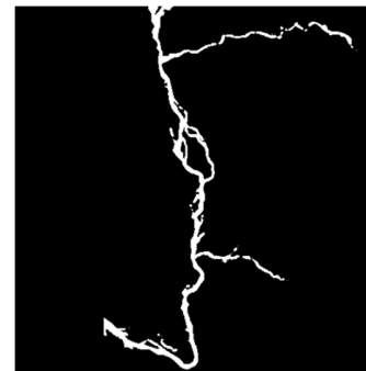
Fig. 2. Derived river map using the combination of MNDWI and AWEI water index.
