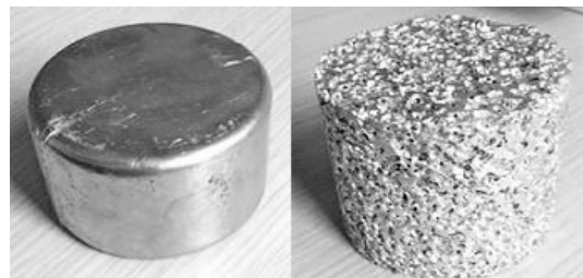
Fig. 1. Aluminum block and resulting foam sample.
