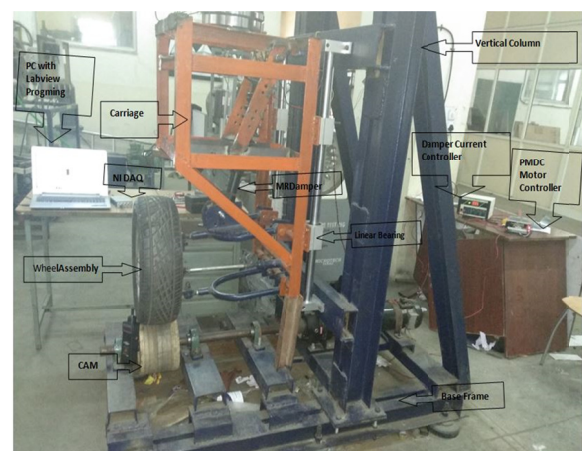
Fig. 3. Experimental setup of quarter car model with MR damper with CS cylinder
