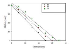
Fig. 4. Relationship between time and oxidized sulfide during oxidation at different sonication intensities.
