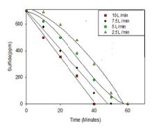
Fig. 2. Relationship between time and sulfide during oxidation at different air flow rates.
