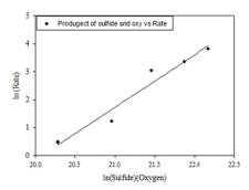
Fig. 5. Linear plot between the product of sulfide concentration and partial pressure of oxygen and rate of sulfide oxidation on logarithmic scale.
