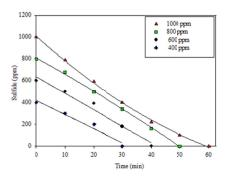
Fig. 3. Relationship between time and oxidized sulfide during oxidation at different initial sulfide concentrations.
