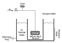
Fig. 1. Experimental set up for the sulfide oxidation in the presence of ultrasonic vibration.
