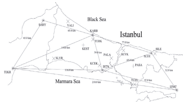
Figure 5. National CORS-TR network geometry with six stations in the study region (*: CORS-TR, +: Rover).
