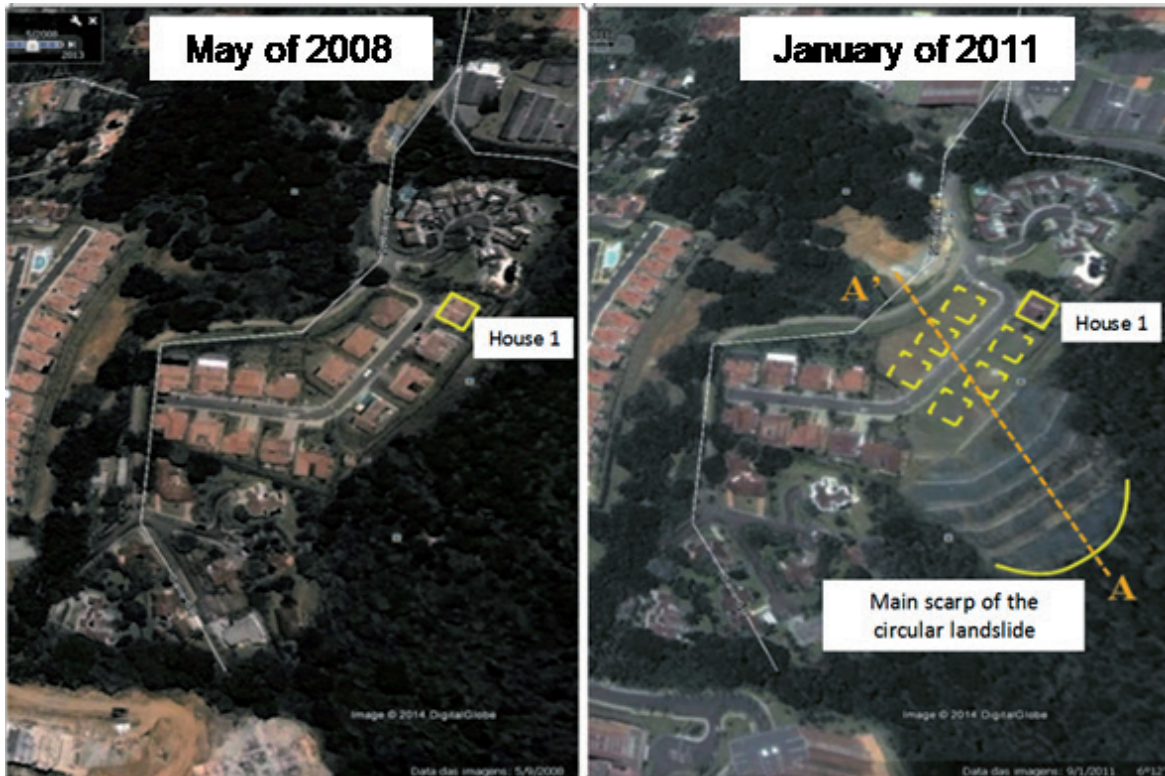
Figure 24. Aerial view of the Alto Verde landslide in 2008 (before) and in 2011 (after). House 1 remains undamaged.
