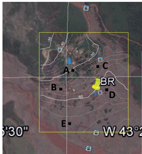
Figure 15. Detailed view of the central part of Bento Rodrigues district and five selected points for analyzing vulnerability. The values indicated on level lines correspond to the difference in height between buildings and dam breaking point.
