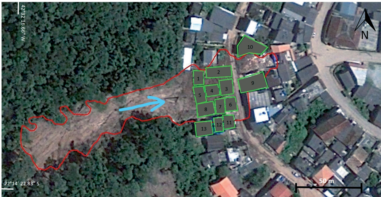
Figure 8. Aerial view of the landslide number 4479 and 13 damaged buildings.
