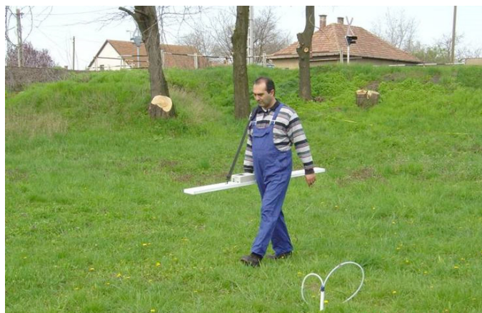
Figure 2. Electromagnetic measurements in the study area using GEM-2 instrument.
