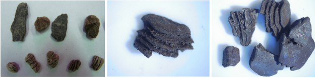
Figure 3. Real cuttings samples selected for creation of specimens.
