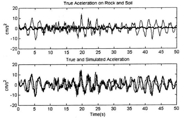
Figure 6. On the top, true acceleration on rock (heavy line) and (soft line) soil. On the bottom, true (soft line) and simulated (heavy line) acceleration for the same time window of soil.
