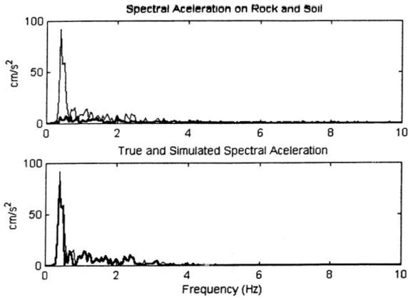
Figure 4. On the top, spectra of soil (soft line) and rock (heavy line). On the bottom, the true (soft line) and simulated (heavy line) spectral acceleration on soil, from learned data.
