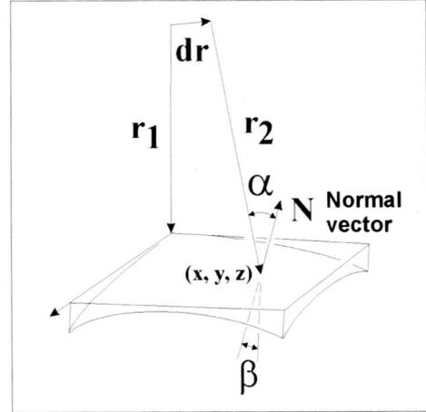
Figure 5. The ray  $\vec{r}_2$  is normal to the next interface in depth, been refracted in  $(x, y, z)$ .  $\alpha, \beta$ : incidence and transmission angles.
