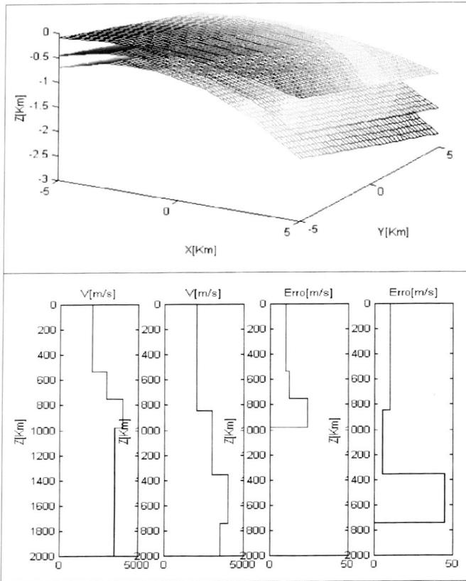
Figure 6. On top the model used to test the algorithm. On bottom interval velocities and erros obtained in two points at the superior surface.
