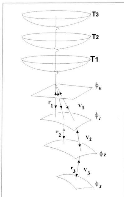
Figure 2. The model is analyzed like three seismic systems, each one with its own central ray and each reflector like its posterior surface. There are travel time functions associated to each system and estimated on the anterior surface (flat).
