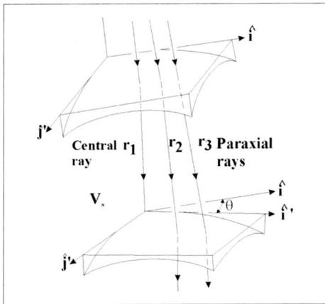
Figure 4. Ray tracing of the central and the paraxial rays through the last solved layer. The new coordinate system  $(\hat{i}', \hat{j}')$  has rotated an angle  $\theta$ .
