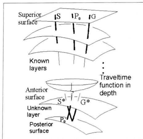
Figure 3. If the sources and detectors were moved from the superior surface to the anterior surface following the ray paths, then the travel time function is determined at the top of the deeper system.
