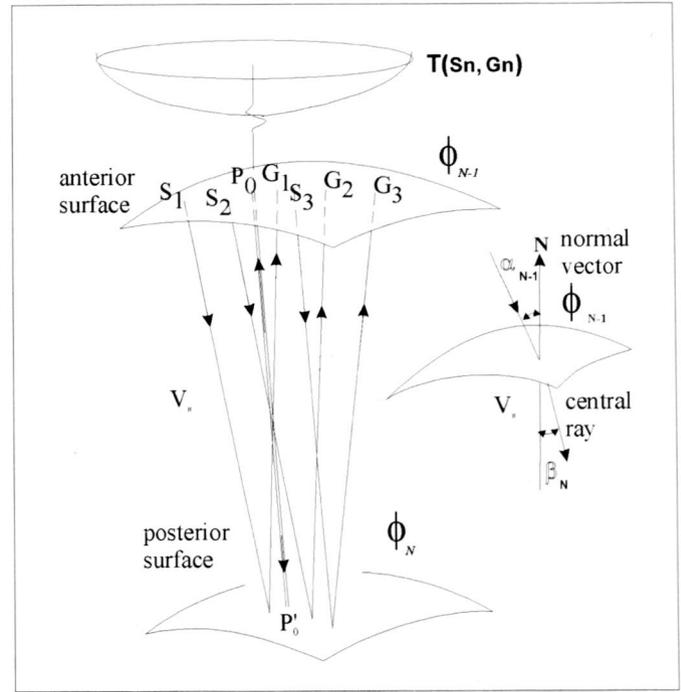
Figure 1. Left: A seismic system and the travel time function of rays reflected on the posterior surface, sources and detectors on the anterior surface. Right: The central ray cross the anterior surface with angles of incidence and transmission.
