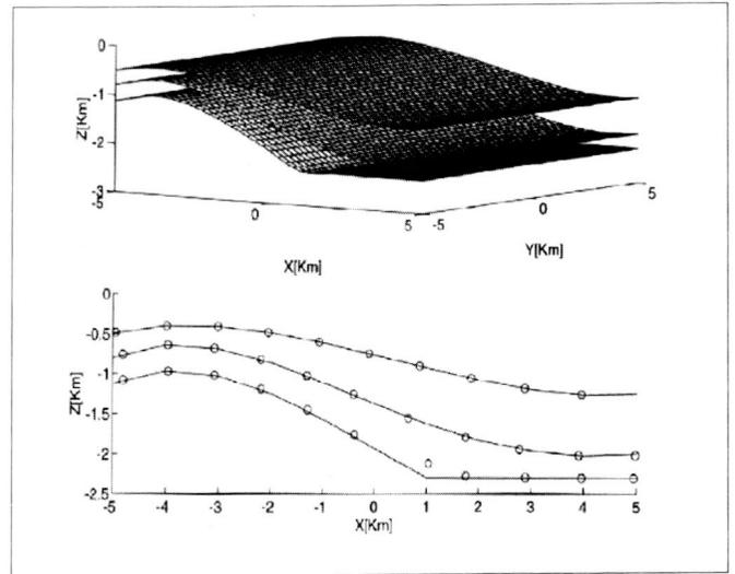
Figure 7. On top the second model and on bottom the interfaces and the points where the algorithm estimates final positions for normal rays.
