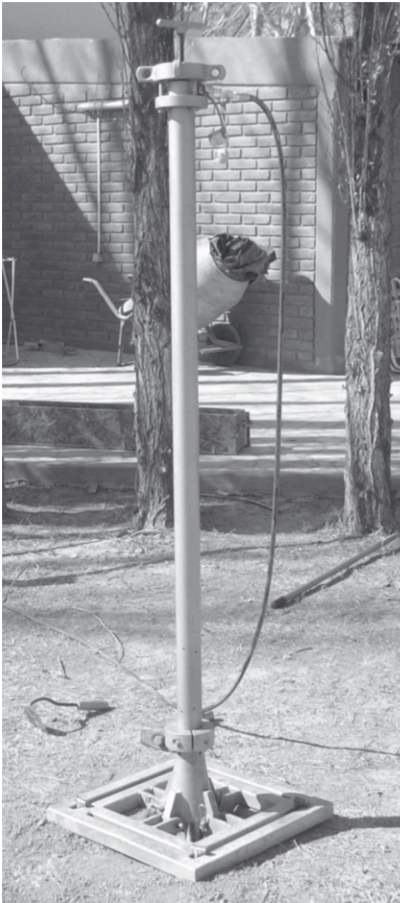
Figure 6. TAMPER. Vertical-Horizontal seismic wave generation system. Vertical implementation.
