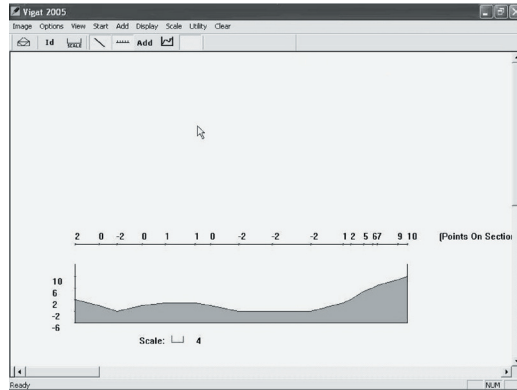
Figure 5. Cross-sections generated by 'Vigat 2005' along section line AA' from Fig. 2 showing variation in gravity data
