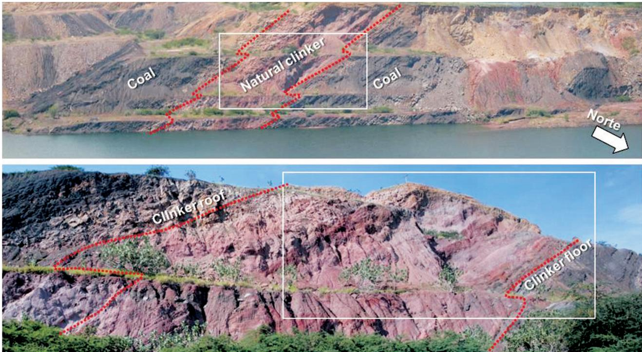
**Figure 1.** Photographs at outcrop scale of natural clinker associated with spontaneous combustion of coal beds, highlighting not only its geometry but also the various shades that present this geologic material.
