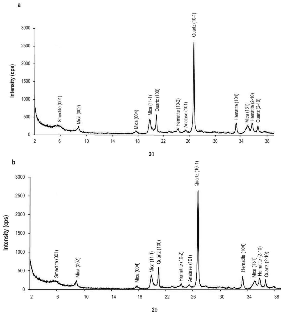
**Figure 5.** XRD patterns of samples NC-1 (a) and NC-2 (b) in the  $2\theta$  range of  $2\text{-}40^\circ$ , using  $\text{Cu-}\alpha.1$  radiation.
