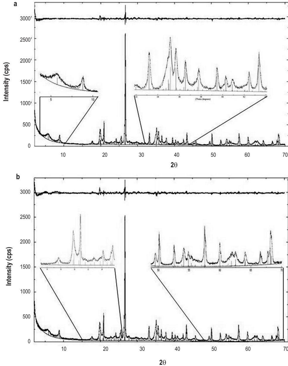
**Figure 7.** XRD profiles refined by the Rietveld method (observed profile in black; calculated profile in red and difference between the observed and calculated profiles in the upper part) from samples NC-1 (a) and NC-2 (b).
