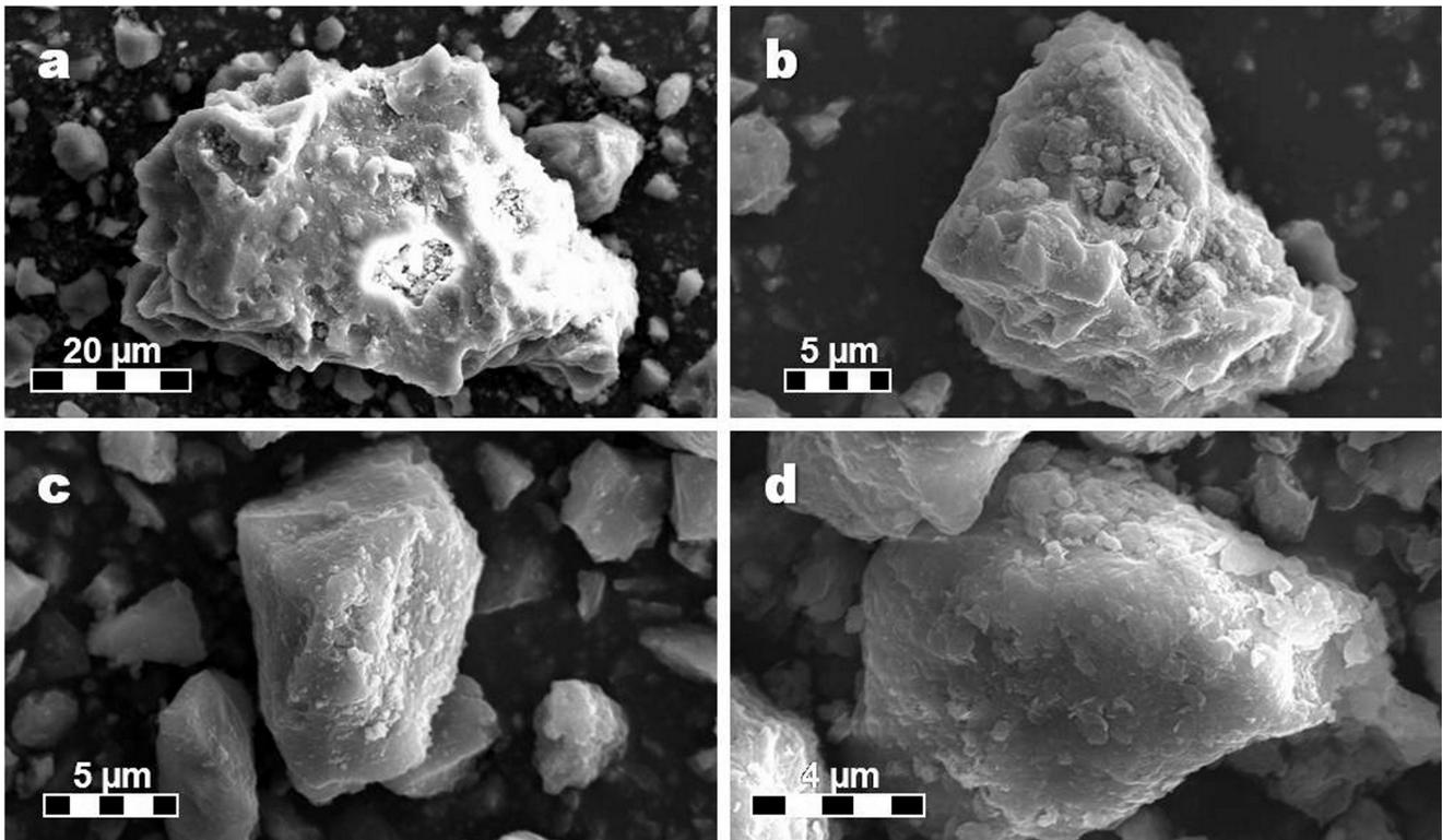
**Figure 4.** SEM images of natural clinker particles.
