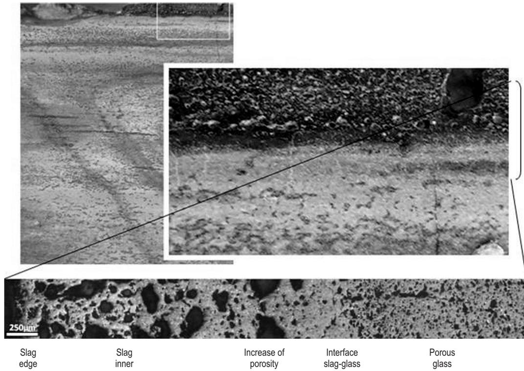
**Figure 3.** Above, photographs of a hand specimen of natural clinker, displaying a vesicular slag appearance. Below, micrograph of the upper left part of the detail shown above. Note the spongy texture and vesicular slag appearance.
