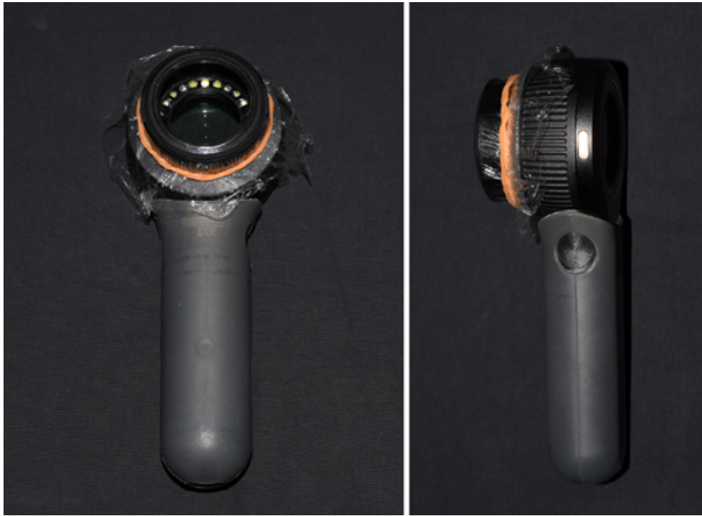
Figure 2. The plastic wrap is firmly stretched over the dermatoscope faceplate then fixed in place with the rubber band.
