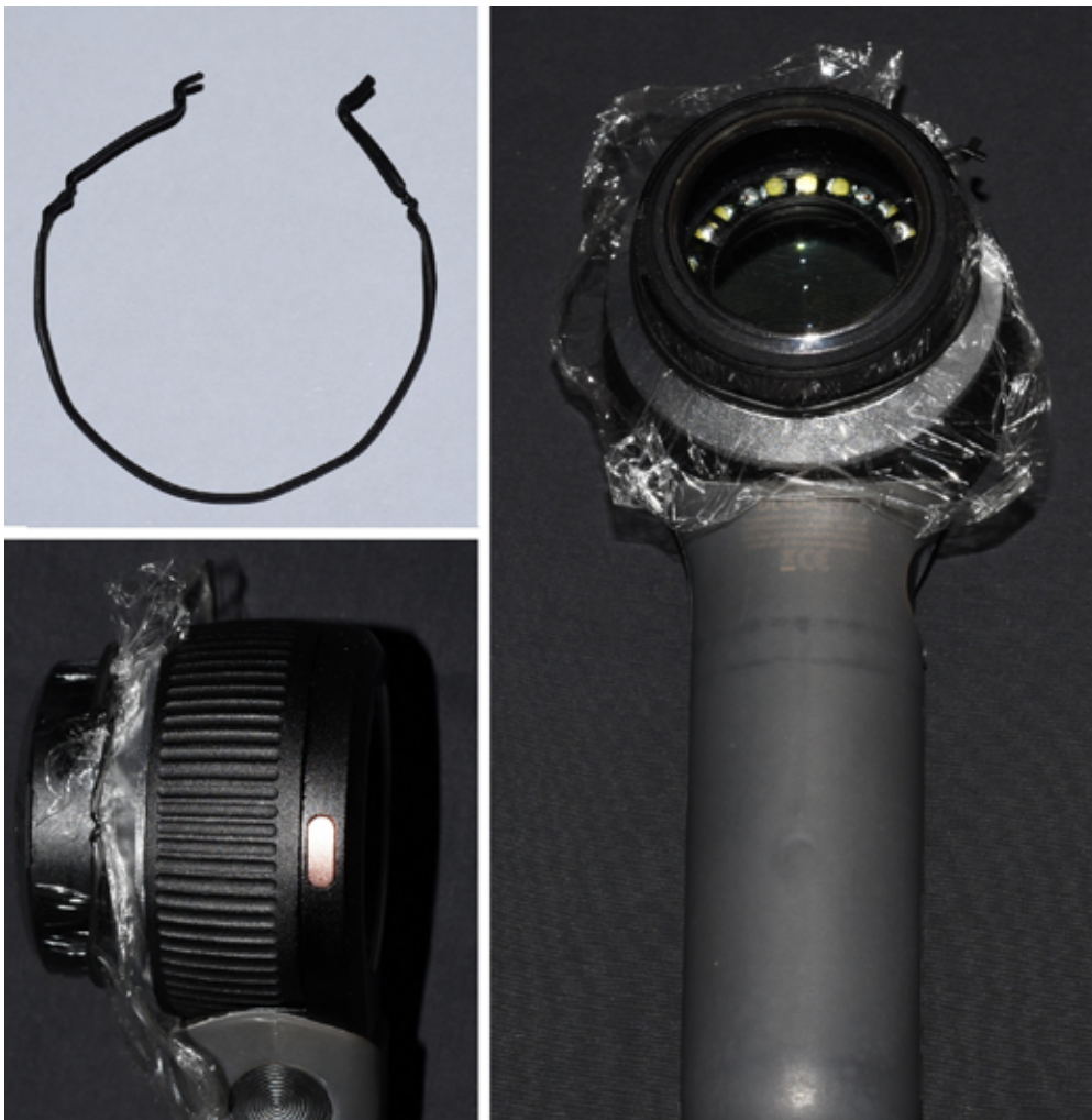
Figure 3. The plastic wrap can also be fixed in place using a metal cable tie.
