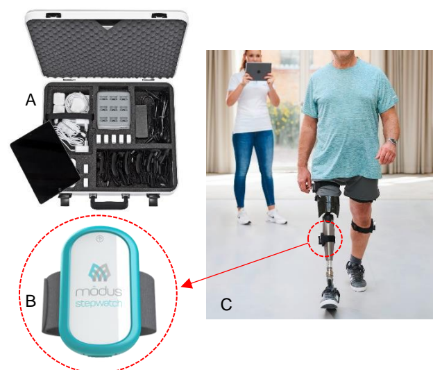
Figure 4: Real real-time sensors to aid in data capture, developed specifically for orthotics and prosthetics are used at Ability as part of daily clinical practice. A: Ottobock Bionic Pro; B: Modus™ StepWatch; C: Real-time, untethered gait analysis being carried out using the Bionic Pro and StepWatch. Persons in image have given informed consent to publication.
