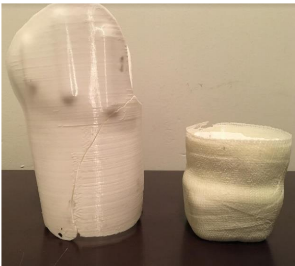
Figure 7: Complete Socket Failure
