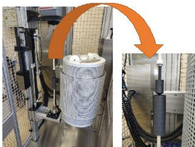
Fig. 3 Internal and external cylinders and the shaft furnace Carbolite STF16/180
