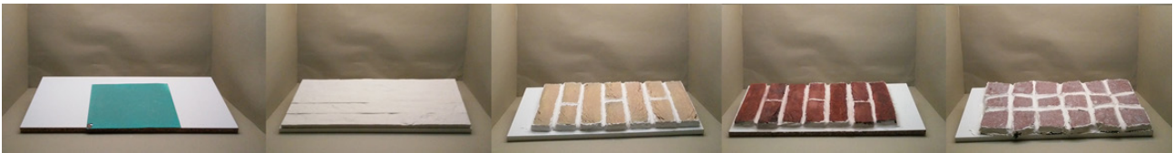
Figure 2 - Selected urban materials for the experiment from left to right: Oxidated Copper Green, Ostuni Natural Stone, Brick Forum Oro, Brick Fermette Cod 160, Porphyry Stone
