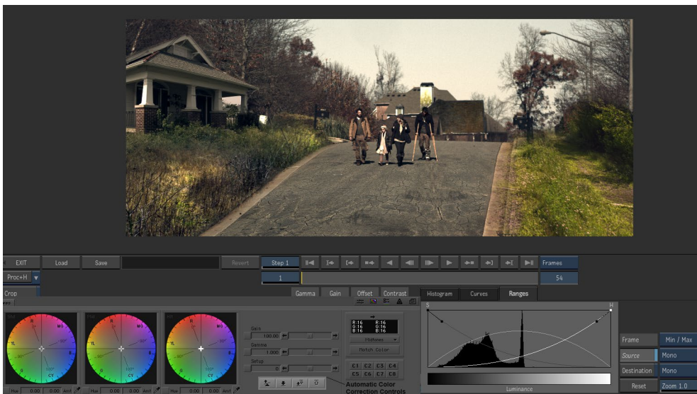
Figure 3 – Example of commercial colour grading software GUI with the main 3-way colour-corrector wheels.
