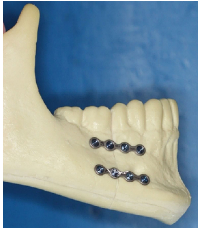
Fig. 1. Group 1: One 2.0 mm mini-plate in the compression zone and another one in the tension zone.
