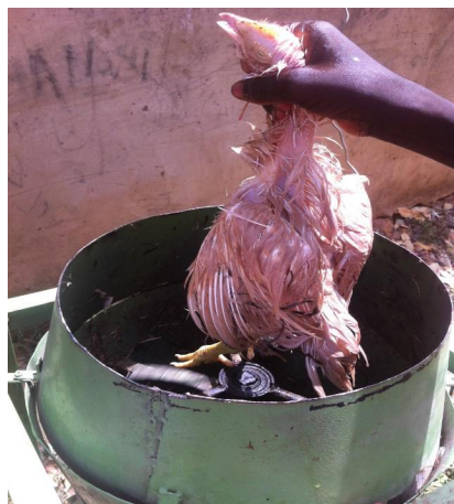
Plate 3: Method of feeding scalded chicken to the machine.
