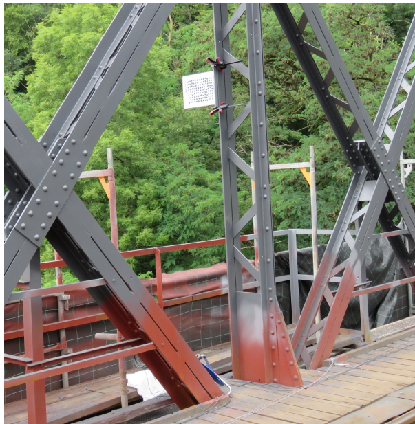
FIGURE 6. The desks with artificial speckle pattern were used to achieve exact location of the tracked points.
