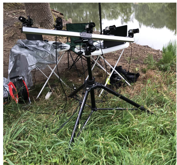
FIGURE 8. The measuring system of the DIC method in the second stage of the experiment.
