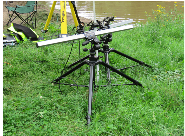
FIGURE 7. The measuring system of the DIC method in the first stage of the experiment.
