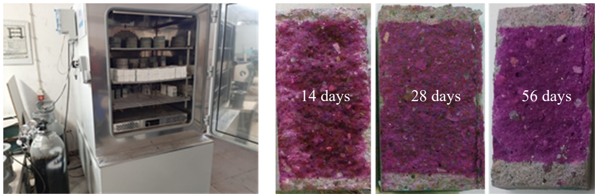
FIGURE 6. Chamber for the carbonation test and evolution of carbonation MT250FA with time.
