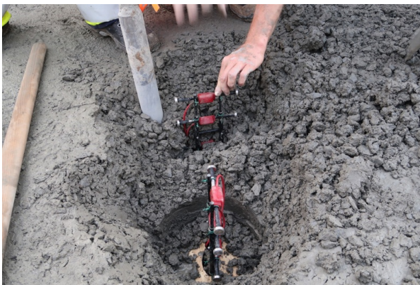
FIGURE 2. Measuring points in the concrete slab.
