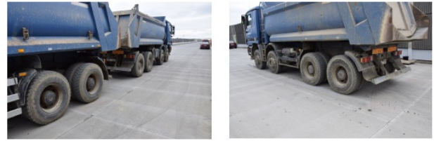
FIGURE 10. Trucks positioning for static load test.
