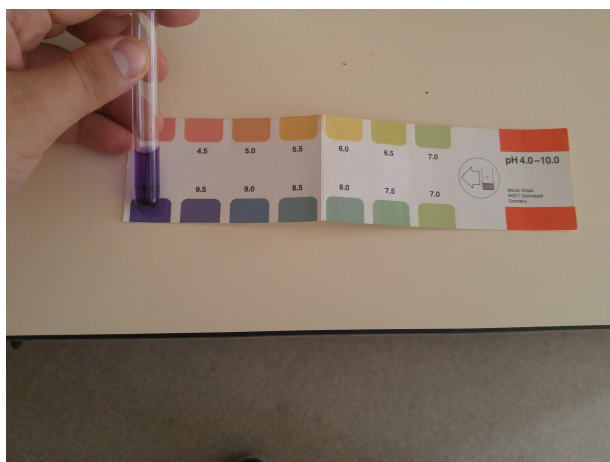
FIGURE 6. Colorimetric evaluation of pH by color and scale.
