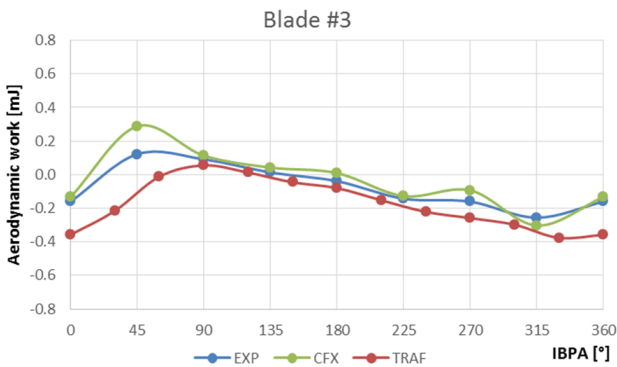
FIGURE 19. Aerodynamic work of blade torsion motion - blade #3: experimental (EXP), CFX and TRAF comparison.
