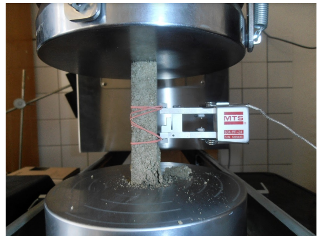
FIGURE 6. Testing of specimens: compressive test.
