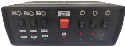
FIGURE 5. Power supply unit - front side.
