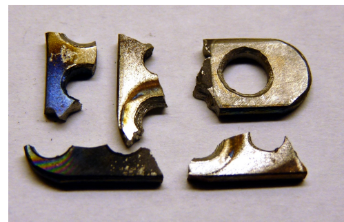
FIGURE 10. Disintegrated cathodes after embrittlement by a hydrogen diffusion into tantalum.
