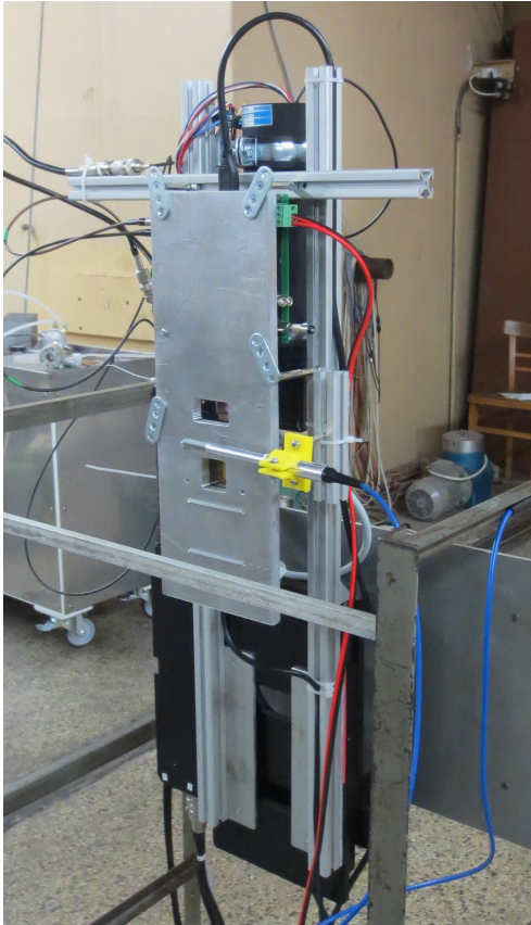
FIGURE 3. Irradiation setup with the Farmer PTW 30010 ionization chamber and the Timepix device.
