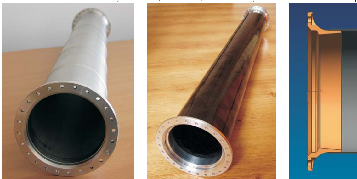
Fig. 1: Driveshaft version 1 (left) and version 2 (center). Detail of connection of flange with central section of versions 2 and 3 (right)
