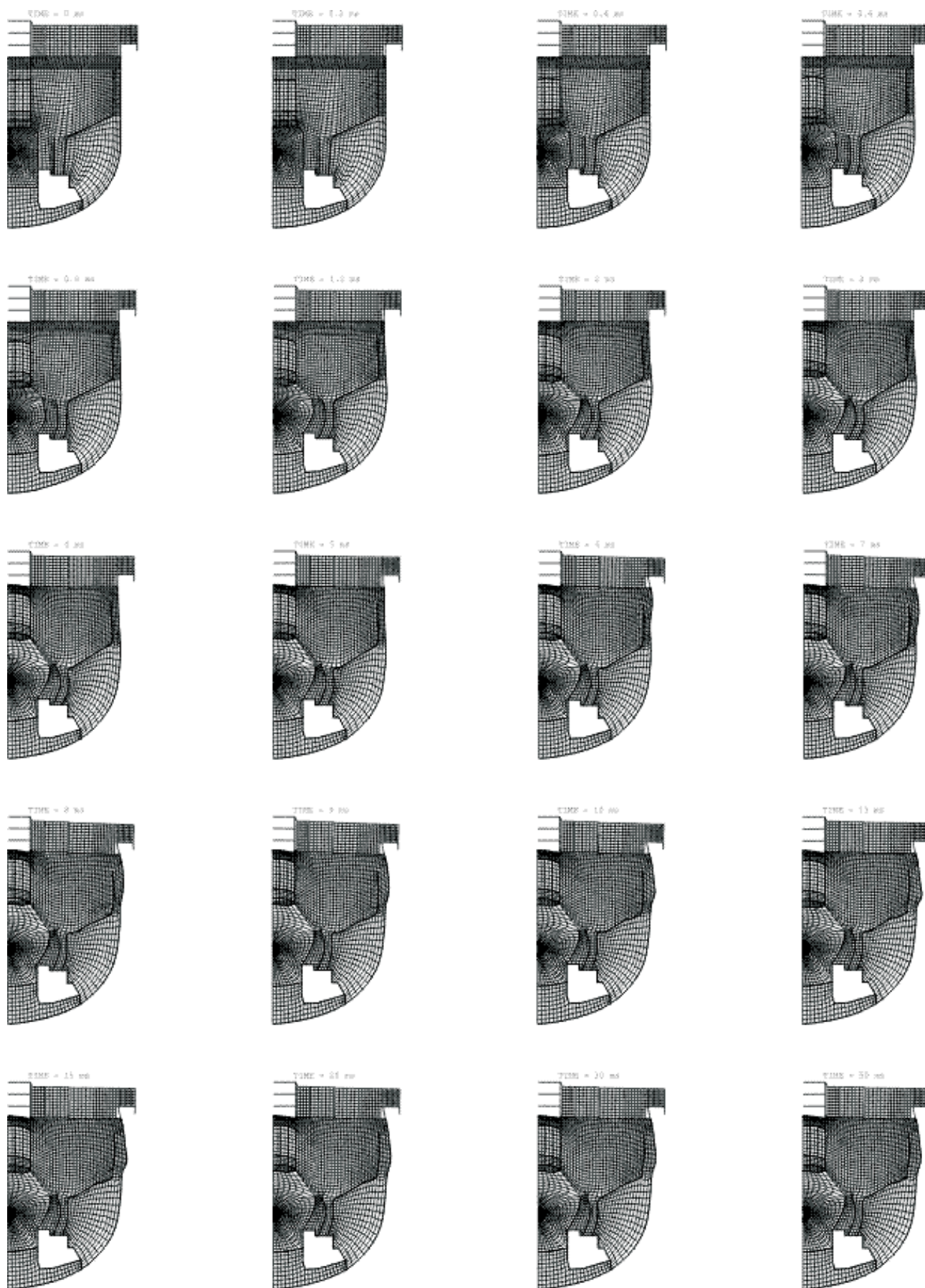
Fig. 13: Deformed shape of the mesh
