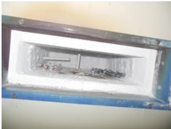
FIGURE 6. Post weld samples in the furnace.
