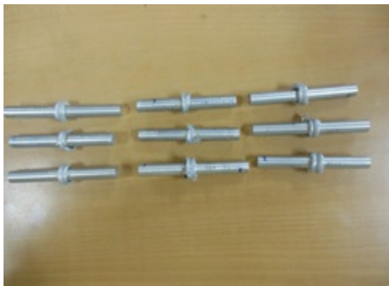
FIGURE 7. Post weld heat treated samples.
