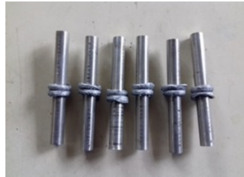
FIGURE 4. Friction welded samples.
