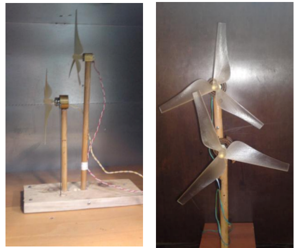
FIGURE 6. Wind turbine models in the wind tunnel.
