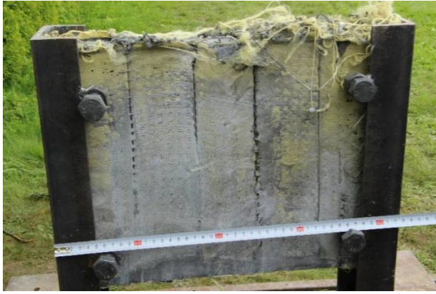
FIGURE 5. Special steel mount with embedded UHP-SFRC thin plate 300 × 400 mm in dimensions with applied Aramid fabrics.
