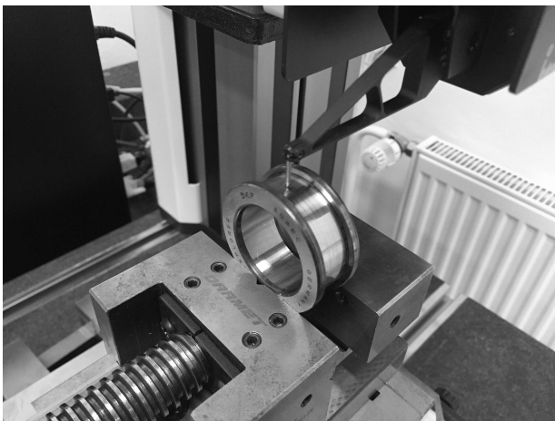
FIGURE 4. Inner race surface texture measurement.
