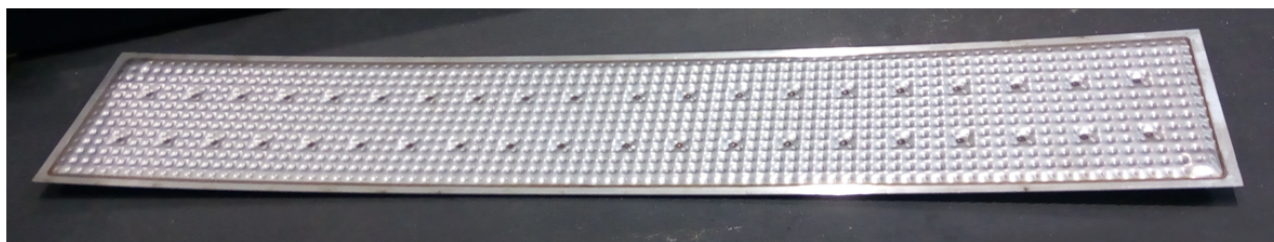
FIGURE 17. Formed solar absorber with the structured surface.
