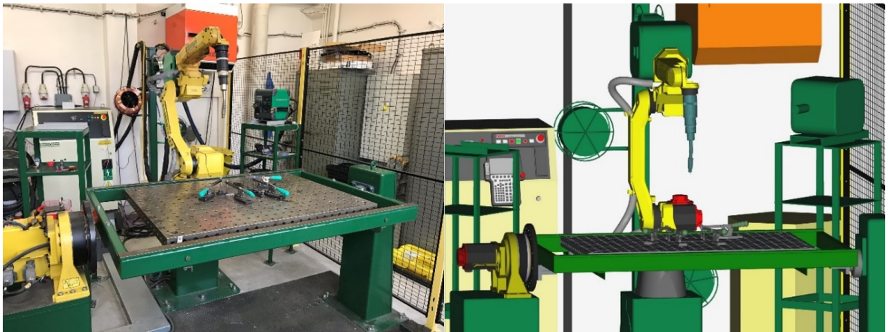
FIGURE 5. View of the real workplace (left), view of the workplace in the FANUC ROBOGUIDE simulator (right).
