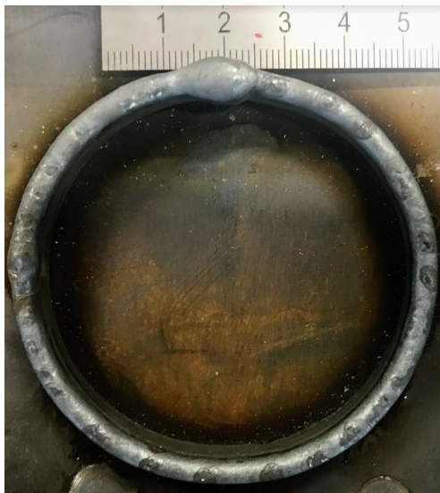
FIGURE 13. Defects caused by too high wire feeding speed.
