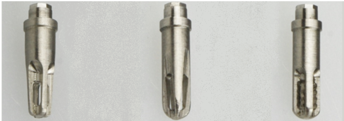
FIGURE 8. All manufactured implant variants. Variant with a conical shape and ribs (left), variant with a system of slant ribs (middle) and variant with a parallel system of ribs (right). All implants have been manufactured from the Ti6Al4V ELI alloy and have a diameter of 3.8mm and length of 8 mm (the most conventionally used size).
