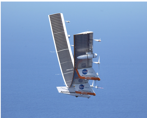
FIGURE 1. The Helios aircraft undergoing large deformation [1].
