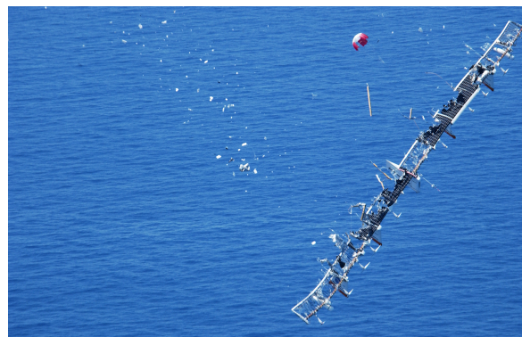
FIGURE 2. The Helios aircraft after structural failure during flight [1]
