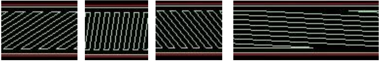
FIGURE 6. Direction of the fibers on different layers of PC specimens – 0 degrees and 90 degrees.
