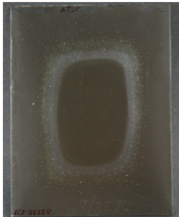
FIGURE 4. Photographic documentation in reflective light of another manifestation of emulsion deterioration which seems like gold micro-spots. Negative Sonneberg 3335.528.
