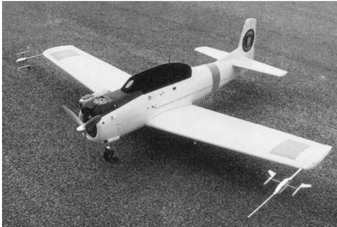
Fig. 5: T28 Trojan instrumented model aircraft
