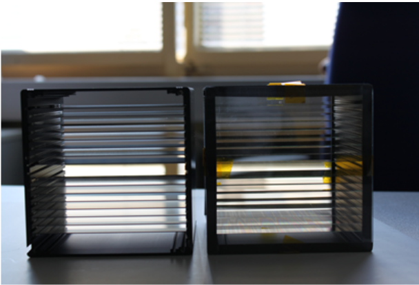
FIGURE 8. Examples of test modules of X-ray MFO optics recently assembled (spring 2012) at RITE in Prague, with both glass foils and silicon mirrors, prepared for full aperture tests at the University of Colorado in Boulder test facility.
