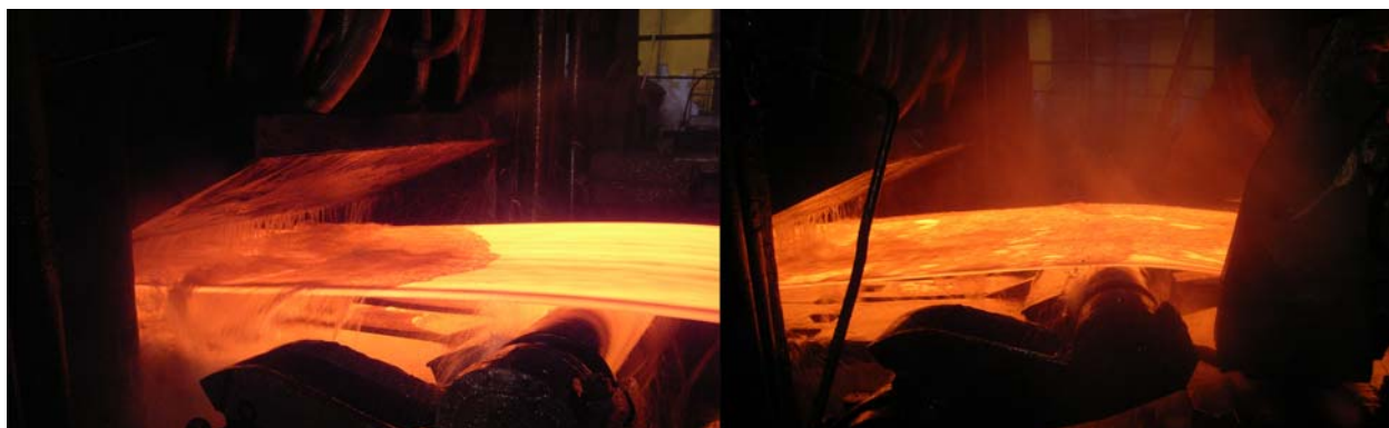
Figure 1: Remnants on the top side of a rolled plate after passing through the cooling section. Although the plate is moving, the water remains on the plate until it evaporates
