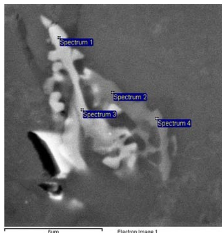
Figure 2: Detail of intermetallic phases of modified structure from electron microscopy and spectral analysis
