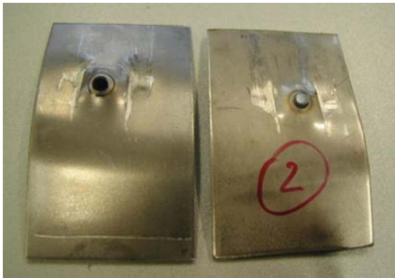
Figure 3: Verification of the weld nugget size (left) and the macrostructure of a selected dissimilar resistance spot weld ( I_W = 7.5 kA)
