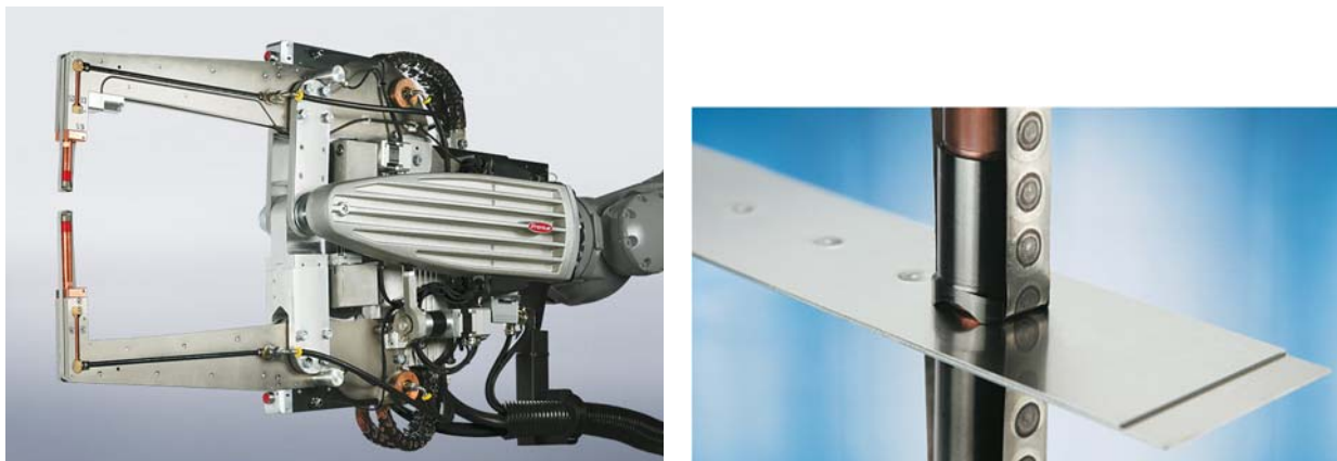
Figure 1: DeltaSpot X-Gun (left) and a detail of the process tapes (right) [5]
