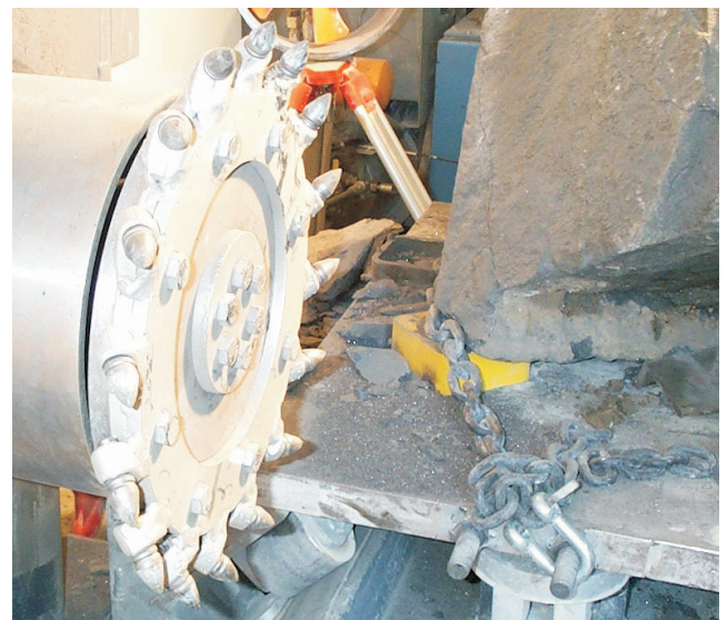
Fig. 1: A typical example of mechanical interaction between bits and hard rock (example of the ore disintegration process)
